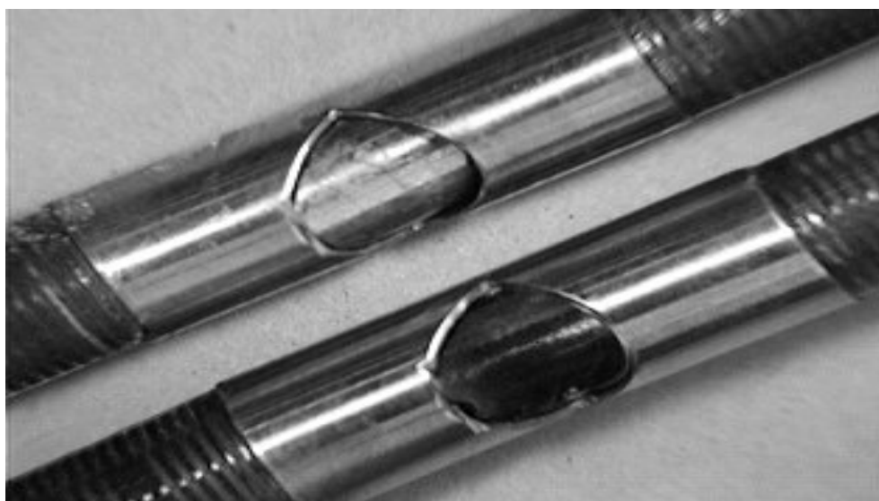
Fig. 1. The combine inflow/outflow valve (patent pending) during aspiration (above) and during ejection (below) used in PUCA-II VAD.
