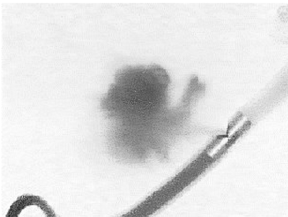
Fig. 4. Flow visualisation during PUCA-II ejection: the ink is ejected under an angle of \pm 45^\circ with the valve housing. The distal part of the catheter is ink free.
